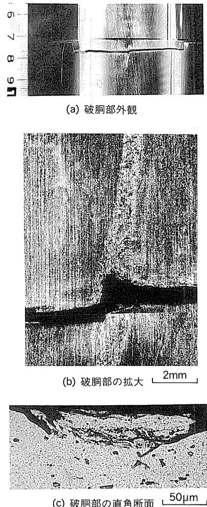
図15 DI缶の破洞 (胴切れ, Tear-off)
