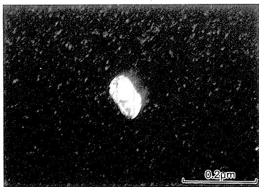
Fig. 7 Precipitation in specimen A intermediately annealed at 473K (and re-annealed at 723K for 10s).
