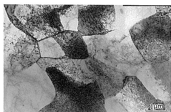
Fig. 11 TEM structure of the specimen B after 50% deformation at  $1 \times 10^{-1}\text{s}^{-1}$ .
