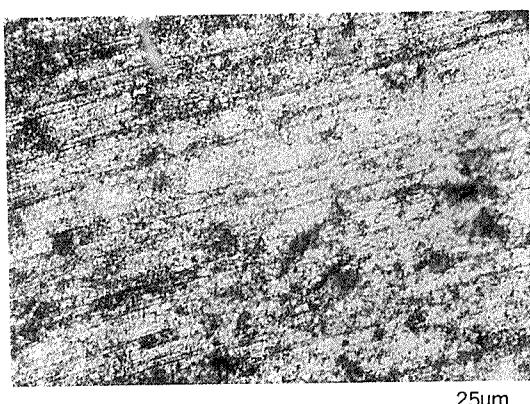
Fig. 5 An optical micrograph of a surface crystal of (Tb,Dy)Fe<sub>2</sub> deformed at 900°C.
