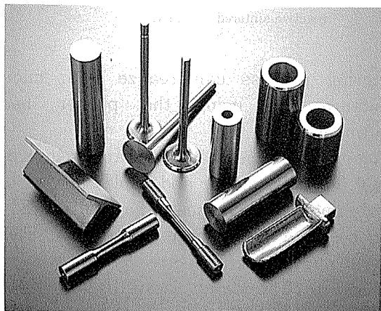
Fig. 4 Samples prepared by reactive-sintering process.
