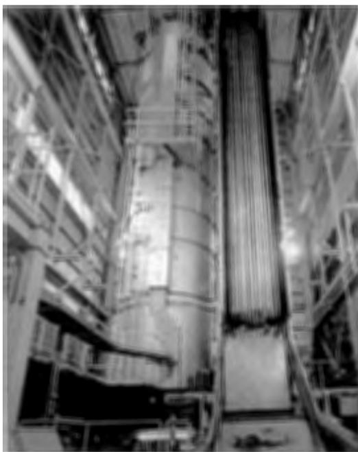
Fig. 11 Vertical quenching furnace.
