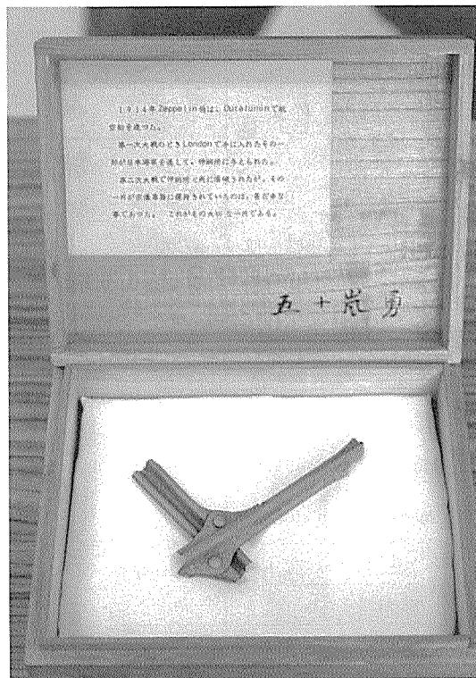
Fig. 12 A piece of Zeppelin's Airship (Duralumin).
