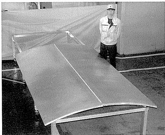
Fig. 17 Large curved shape of brazed honeycomb panel produced by friction stir welding.
