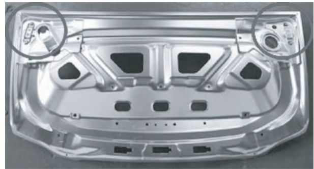
Fig. 8 FSSW of aluminum to steel used in an aluminum trunk lid 13) .
