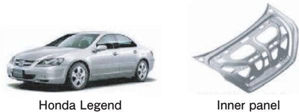
Fig. 8 Automotive parts for QPF of aluminum alloys<sup>9)</sup>.
