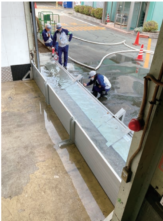
Fig. 2 Flood barrier testing at our own facilities. It was not a complete watertight seal, but only a small amount of water leaked.
