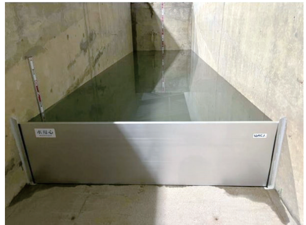
Fig. 3 Flood barrier testing at 450mm water height at Kyoto University facilities.
