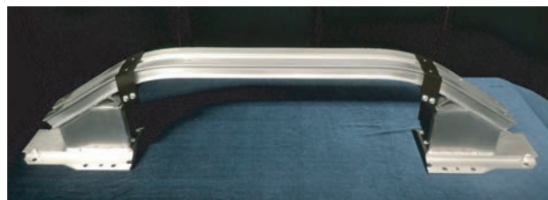
(a) Hollow section bumper reinforcement.
