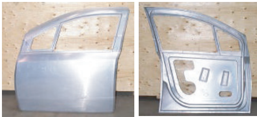
Fig. 10 Panel formed by QPF 10) .
