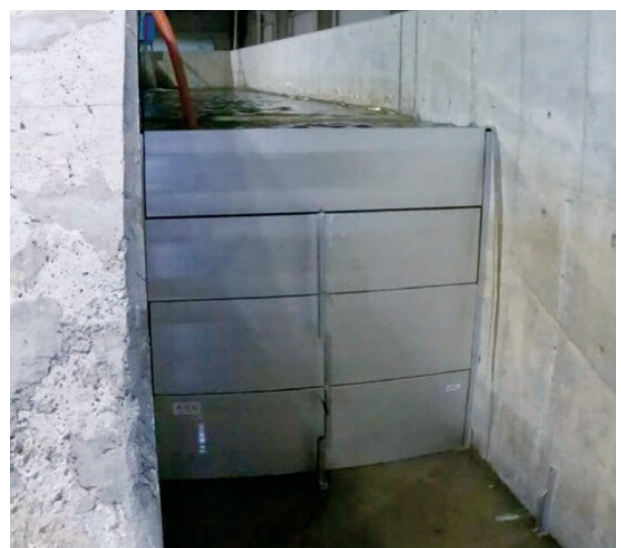
Fig. 4 Strength evaluation at 2,000 mm water height at Kyoto University facilities.
