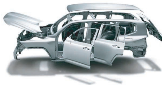
Fig. 1 White body of Toyota Land Cruiser.
