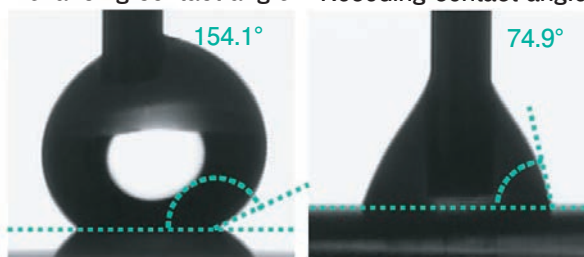
Fig. 12 Appearances of water droplets on (a) the PEO film formed by galvanostatic anodizing of high-purity Al at 100 \text{ Am}^{-2} in 0.9 M ammonium tetraborate solutions at 323 K for 60 min during a static contact angle measurement and (b) the HDFOPA-SAM-coated PEO film during a dynamic contact angle measurement.
