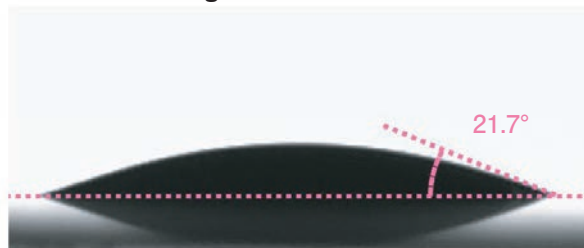
(b) PEO film after SAM coating Advancing contact angle Receding contact angle
