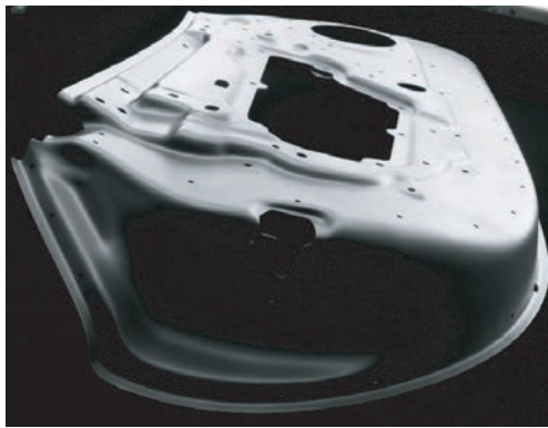
Fig. 14 Application example of HFQ (Inner door panel) *1) .
