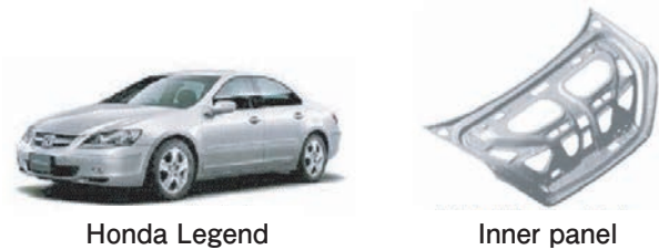
Fig. 8 Automotive parts for QPF of aluminum alloys 9) .
