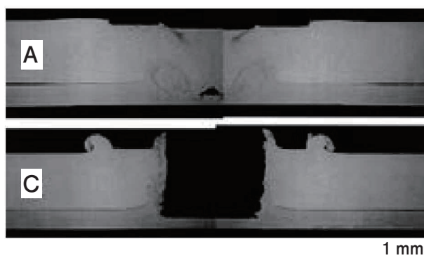
Fig. 13 Microstructure of adjustable (A) and conventional (C) FSSW joints in 3 mm/1 mm sheet thickness 12) .
