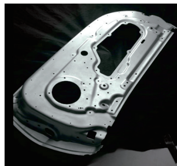
Fig. 19 Products (high strength 6000 series alloy) formed by hot stamping (HFQ ® ) 25) .
