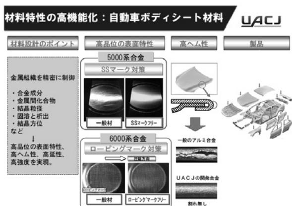
Fig. 6 Aluminum alloys for automotive body panels.
