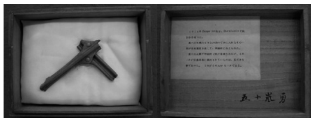
Fig. 10 Part of framework of Zeppelin Airship shot down in near London, brought into Japan by Japanese Navy and the authentication of Dr. Igashiki on the box stored in UACJ Corporation 10)
