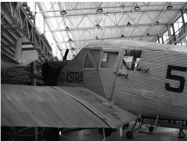
Fig. 8 Junkers F.13 was the world's first all-metal transport aircraft fabricated with corrugated panels of Duralumin sheets, developed in Germany at the end of World War I. ( http://www.idflieg.com/junkers-fl13.htm , ©2006 Andi Szekeres)
