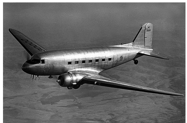
Fig. 12 DC-3 fabricated with Alclad 24-T3 sheets. http://www.boeing.com/boeing/history/mdc/dc-3.page
