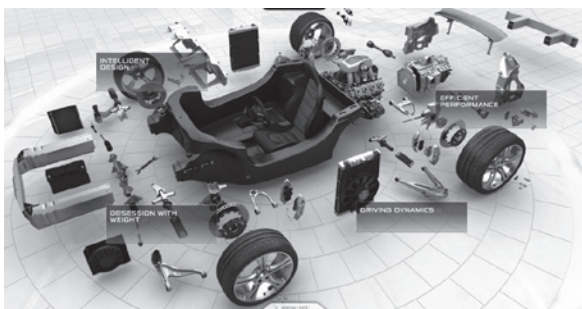
Fig. 16 Dissimilar material bodies of CFRP center cabin with aluminum parts of McLaren MP4-12C.
