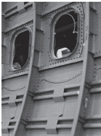
Fig. 8 B767's fuselage constructed with frames, skins and taper-rolled stringers (left). Manufacturing process of a taper-rolled stringer for airplanes (right) 17) .
