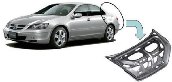
Fig. 16 High-temperature blow-formed trunk lid inner of the Honda Legend<sup>23)</sup>.
