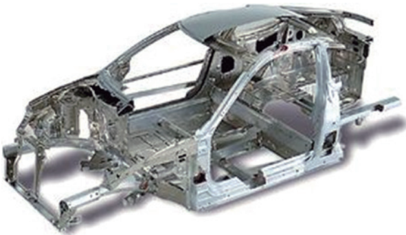
Fig. 3 Aluminum space frames structures of HONDA Insight 6) .
