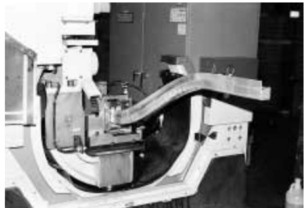
Fig. 4 Push-through bending on HONDA Insight 6) .
