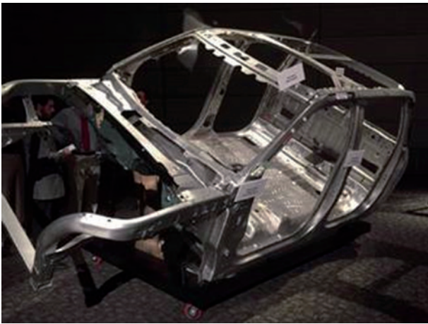
Fig.11 Hydro forming on FORD F-150.
