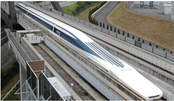
Fig. 10 The linear motor train made from aluminum alloy panel structure which has been welded by FSW method.
