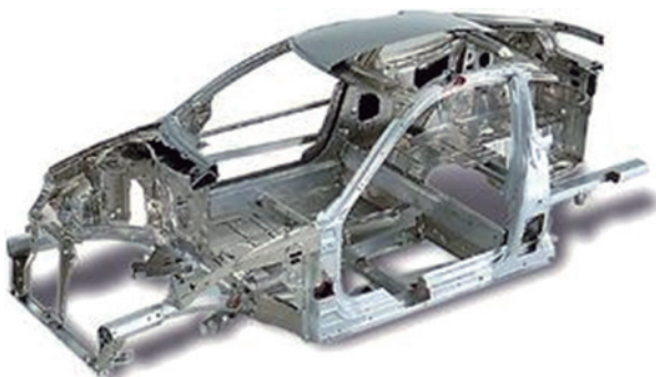
Fig. 3 Aluminum space frames structures of HONDA Insight 6) .
