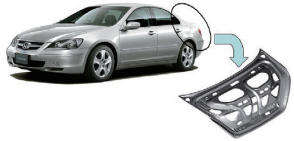
Fig. 16 High-temperature blow-formed trunk lid inner of the Honda Legend 23) .
