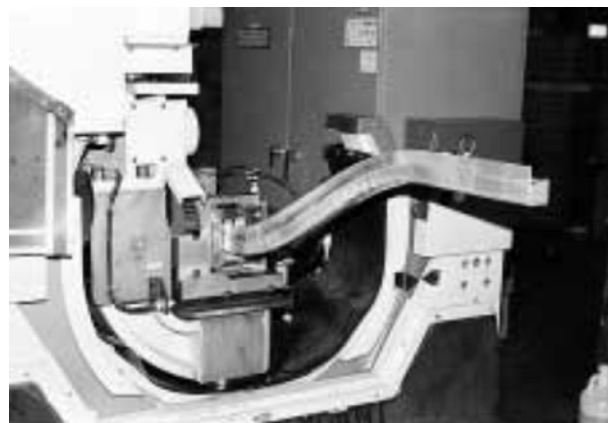
Fig. 4 Push-through bending on HONDA Insight 6) .
