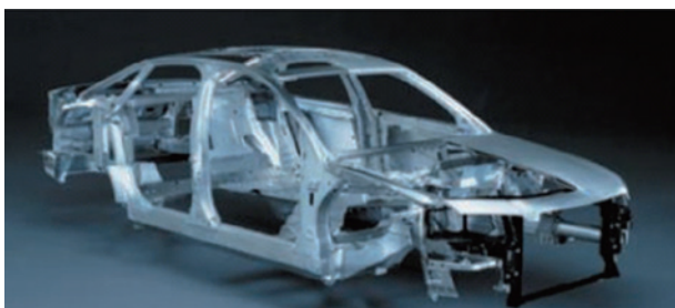
Fig. 16 Space frame structure vehicle (A8/Audi) 8) .
