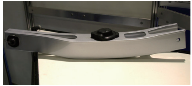
Fig. 8 Suspension arm of Suzuki KIZASHI made of extrusion (2010).
