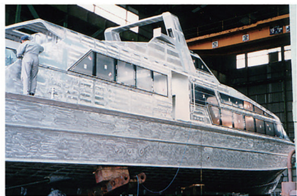
Fig. 7 5083-aluminum alloy panels used in the superstructure of the ship which was stiffened by PRERIB®.
