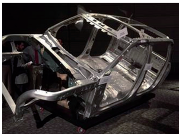
Fig.11 Hydro forming on FORD F-150.
