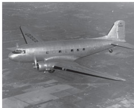
Fig. 5 DC-3 fabricated with Alclad 24S-T3 sheet<sup>14)</sup>.
