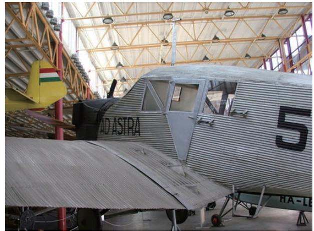
Fig. 3 Junkers F.13 fabricated with corrugated panels of Duralumin sheets (©2006 Andi Szekeres) <sup>9)</sup>
