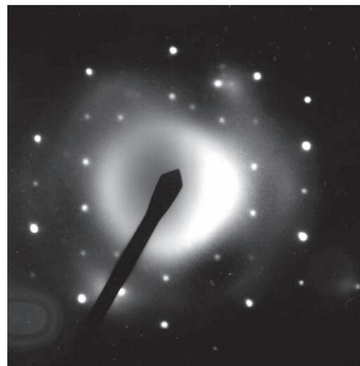
Fig. 5 SAD pattern observed in the specimen prepared with the intermediate annealing at 473 K.
