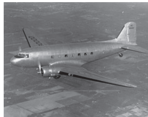
Fig. 5 DC-3 fabricated with Alclad 24S-T3 sheet 14) .
