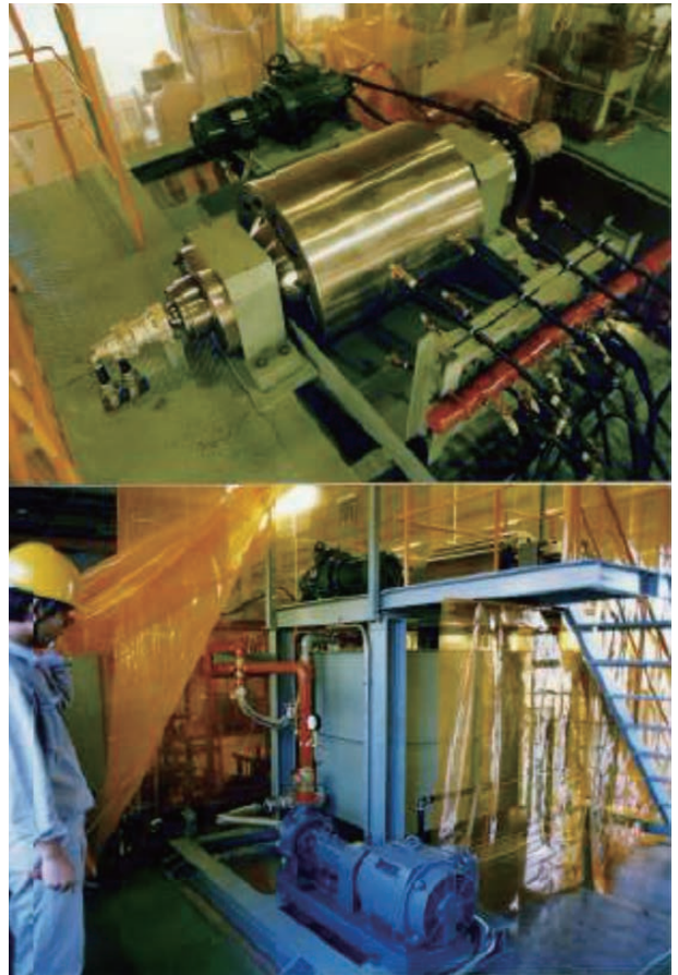
Fig. 47 Experiment apparatus to evaluate the roll cooling 25) . (upper: roll and the spray nozzles, lower: coolant tank)
