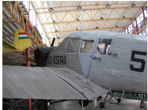
Fig. 3 Junkers F.13 fabricated with corrugated panels of Duralumin sheets (©2006 Andi Szekeres) 9)
