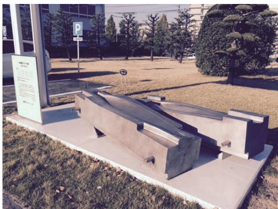
Fig. 11 Forging die of propellers for Zero Fighter stored in UACJ Corporation, Nagoya.
