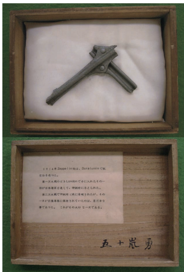
Fig. 1 Part of the frame of Zeppelin Airship crashed near London, brought into Japan by Japanese Navy and stored in UACJ Corporation 1) .
