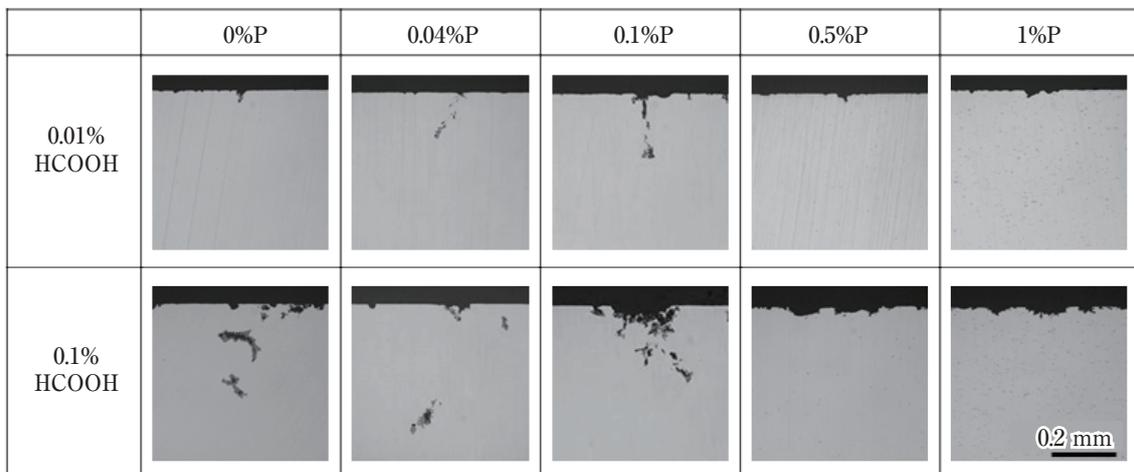
**Fig. 3** Maximum corrosion depth of the copper alloy tubes after 20 days exposure to 0.1% formic acid vapor as a function of phosphorus content.
