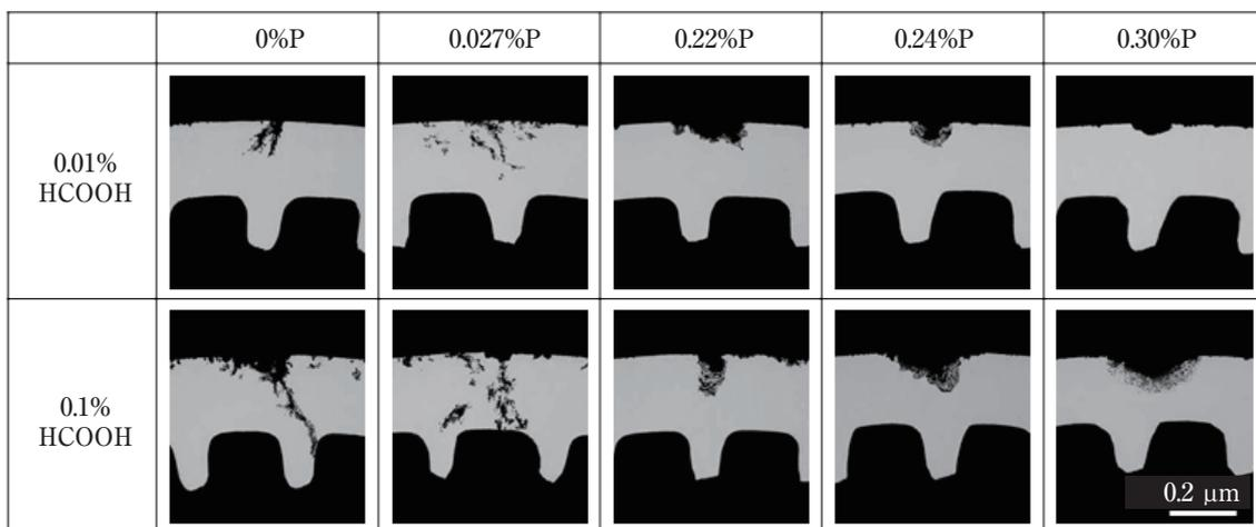
**Fig. 7** Cross-sectional images of the deepest corrosion pit occurred on various copper tubes after 80 days exposure to 0.01 or 0.1% formic acid vapor.
