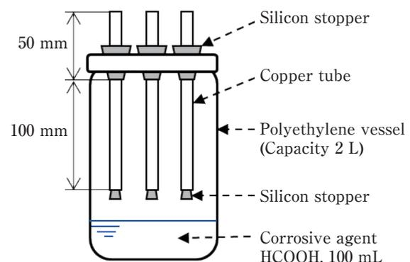
**Fig. 1** Schematic diagram of the corrosion test cell.
