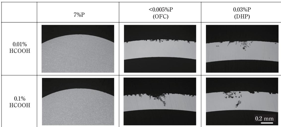
**Fig. 2** Cross-sectional images of Cu-7mass%P, Oxygen free copper and Phosphorus deoxidized copper tubes after 80 days exposure to 0.01 or 0.1% formic acid vapor.
