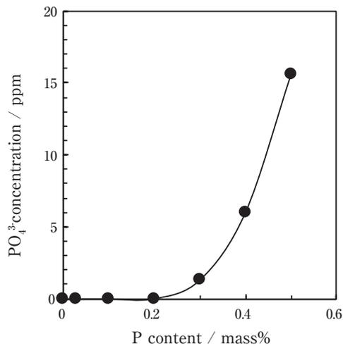
**Fig. 8**  $\text{PO}_4^{3-}$  concentration dissolved from the copper alloy chips as a function of phosphorus content.
