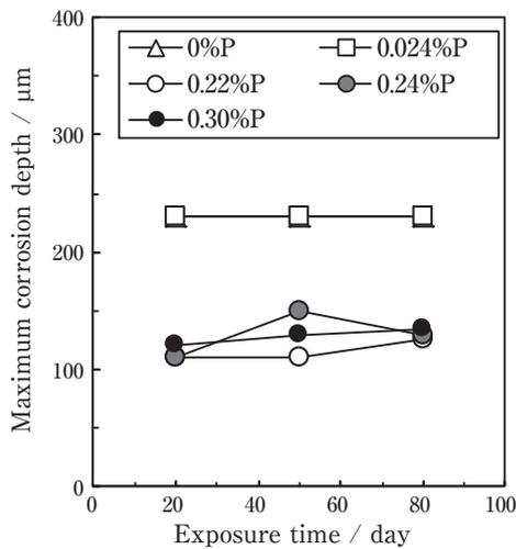
**Fig. 6** Maximum corrosion depth of various copper tubes as a function of exposure time to 0.1% formic acid vapor.
