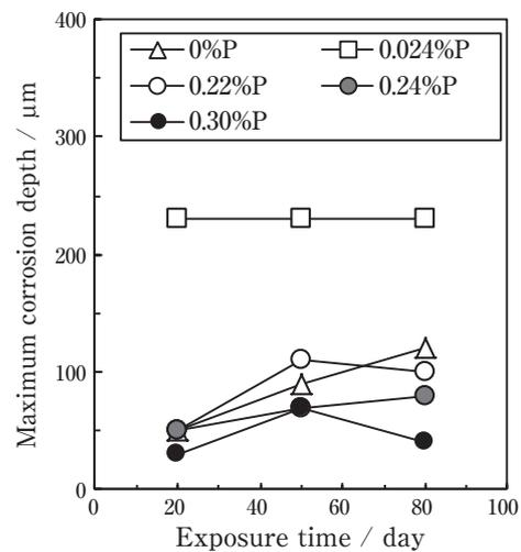
**Fig. 5** Maximum corrosion depth of various copper tubes as a function of exposure time to 0.01% formic acid vapor.
