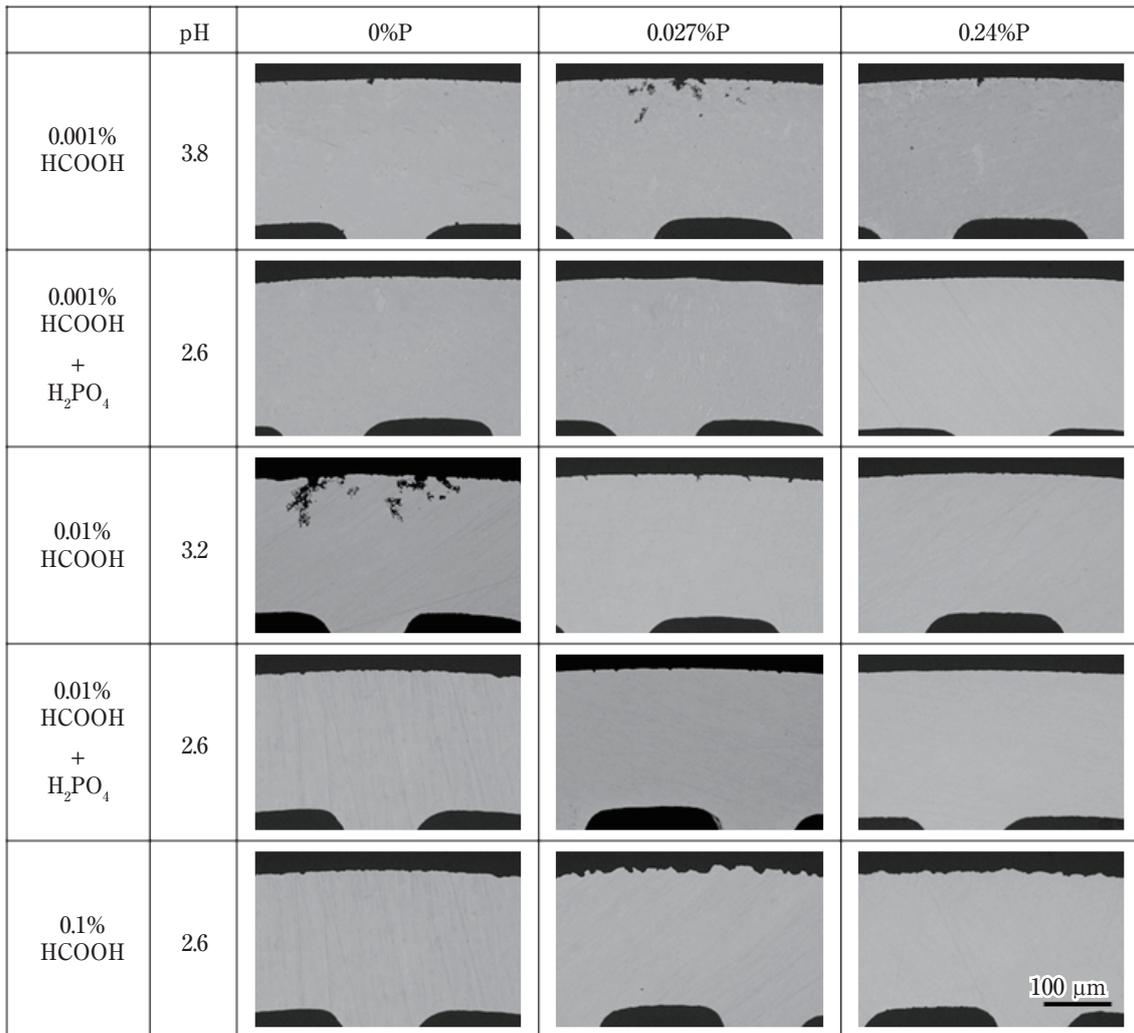
**Fig. 9** Cross-sectional images of the deepest corrosion pit occurred on various copper tubes after 80 days exposure to 0.01 or 0.1% formic acid vapor.
