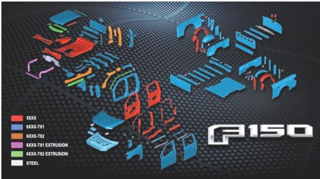
Fig. 1 Material selection for each part of the upper body for Ford F150.
