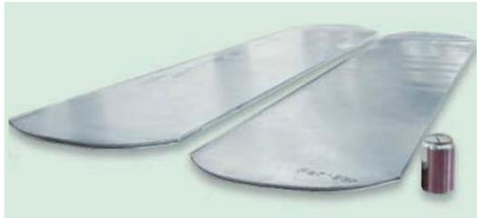
Size comparison between the rolled alloy sheet (TS : 735MPa, YS : 687MPa, EL : 10%) of 450 mm width and a beverage can.
