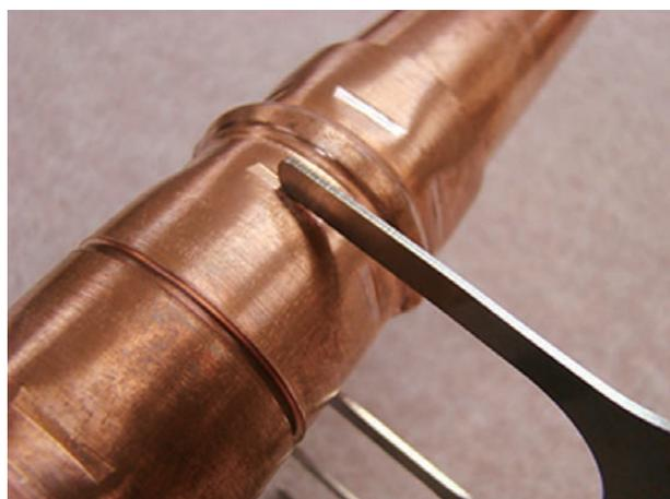
Fig. 8 Press-crimping quality check using the specialized gauge.
