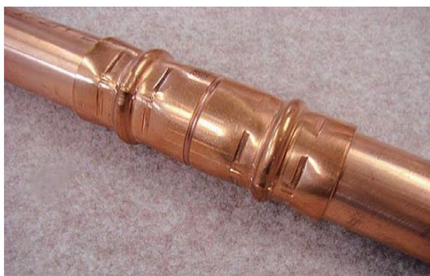
Fig. 7 Appearance of RG-press after the press-crimping.
