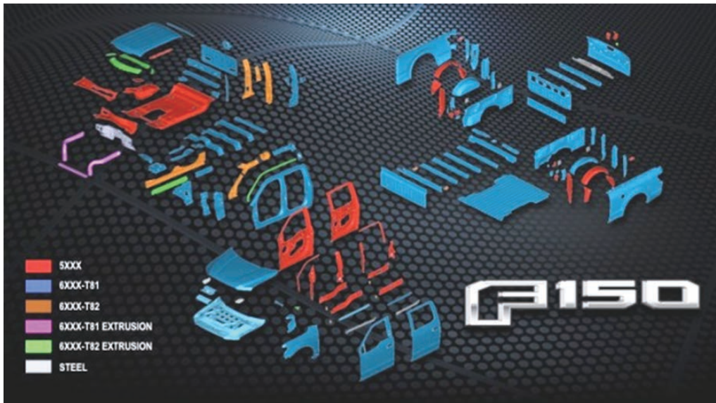
Fig. 1 Material selection for each part of the upper body for Ford F150.
