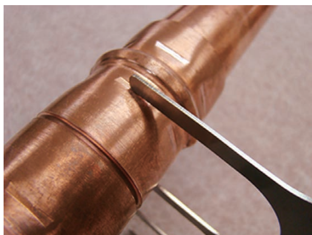
Fig. 8 Press-crimping quality check using the specialized gauge.
