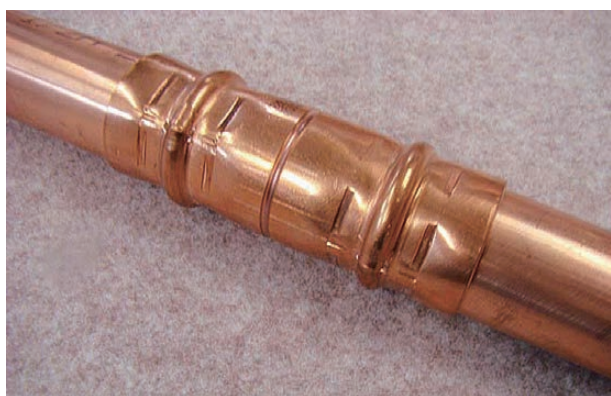
Fig. 7 Appearance of RG-press after the press-crimping.
