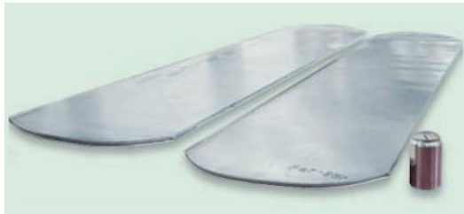
Size comparison between the rolled alloy sheet (TS : 735MPa, YS : 687MPa, EL : 10%) of 450 mm width and a beverage can.
