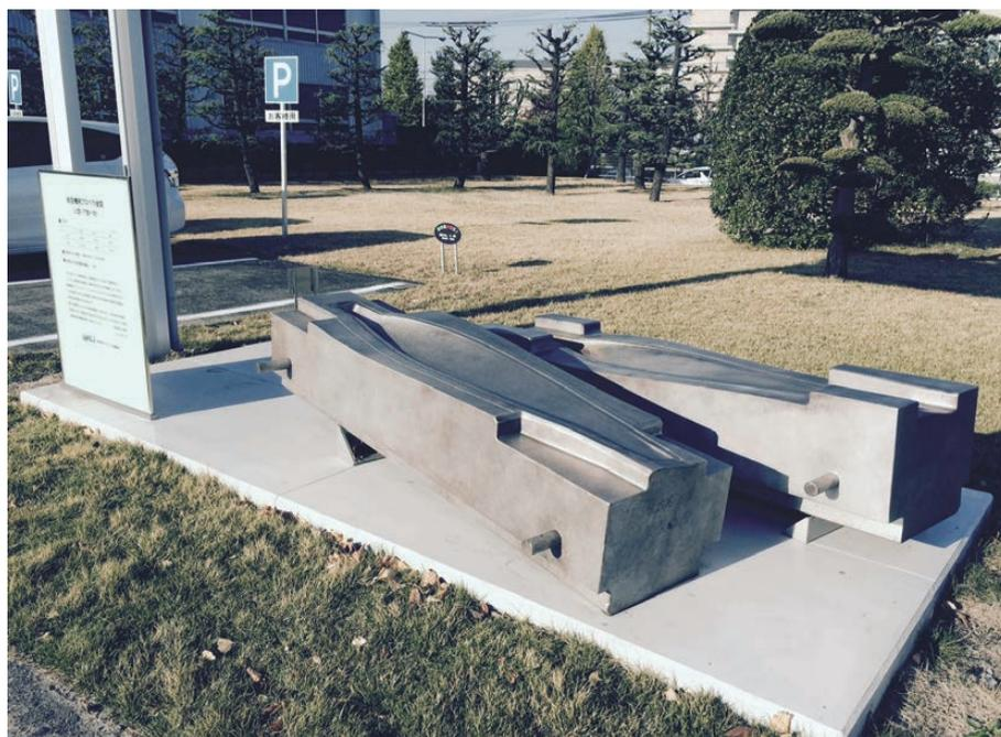
Fig. 9 Aircraft propeller dies (upper and lower dies pair) displayed at the front entrance of UACJ Corporation, Nagoya Works.
