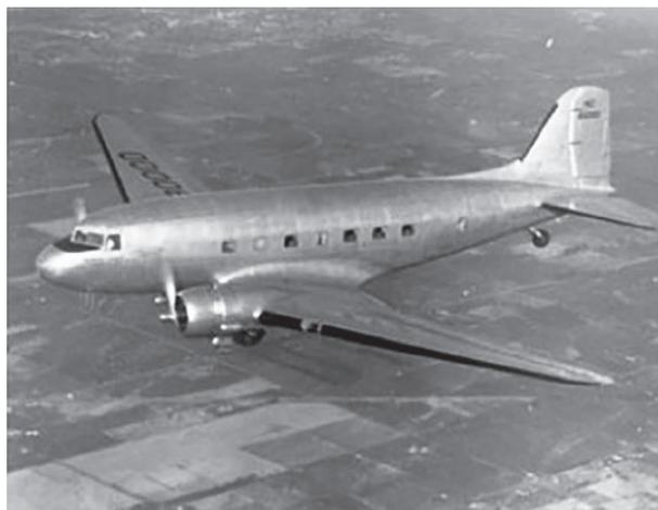
**Fig. 2** DC-3, the first aircraft to use Alcoa's Alclad 24S-T3 on the fuselage<sup>20)</sup>.
