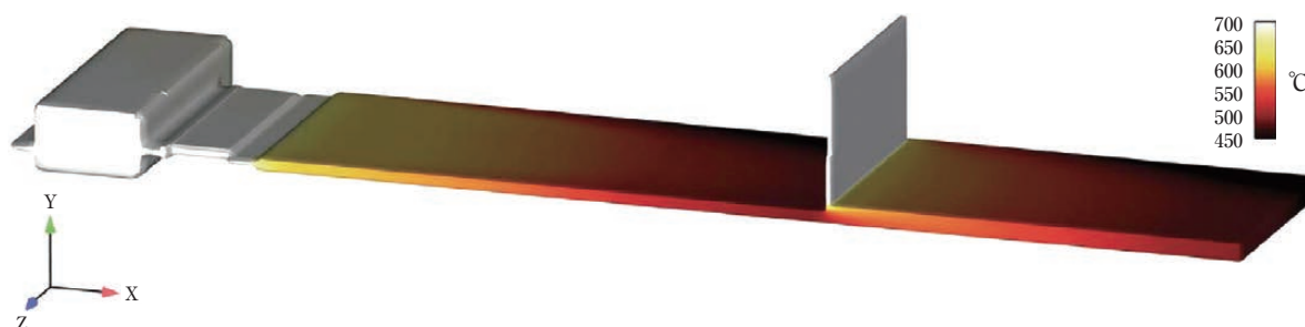
Fig. 15 Clad materials temperature distribution in belt caster. 46)
