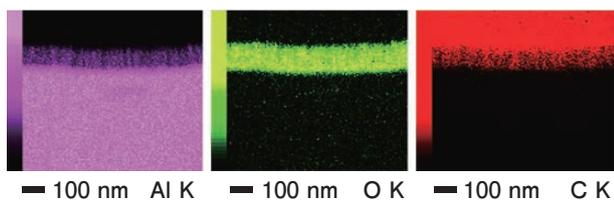
**Fig. 7** Composition mapping of the aluminum/resin interface.
